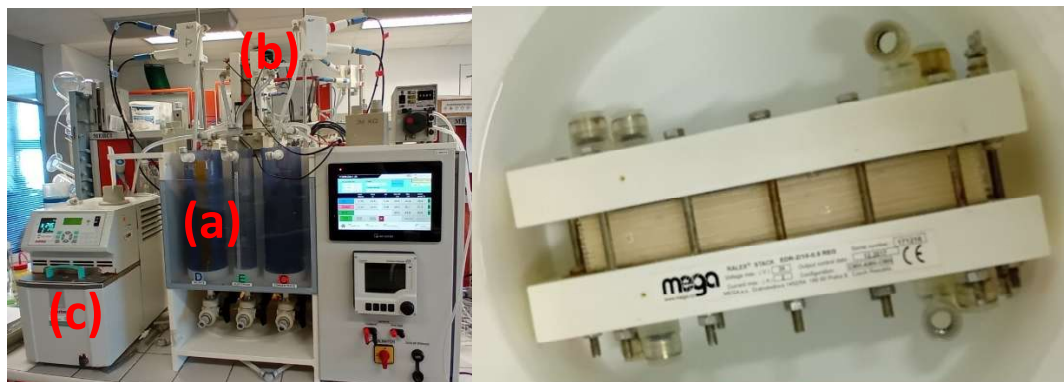
Figure 1 Left: P EDR-Y elektrodialysis unit (a) with membrane (b) and temperature control (c), Right: membrane module
